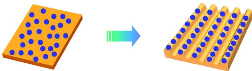
FIGURE 4 Schematic illustration of patterning of functional materials via the conveyance actions of photo-triggered mass migration in the Az polymer film.
